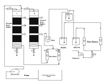
Fig. 1 Schematic diagram of biofilter
