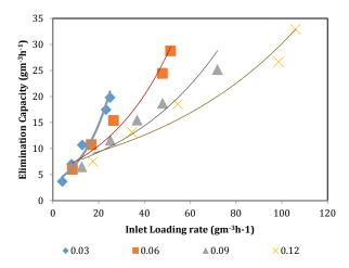
$\textbf{Fig. 6} \ Inlet \ Load \ Vs \ Elimination \ capacity \ for \ the \ removal \ of \ MEK \ using \ Press \ mudbased \ biofilter$
