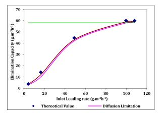
Fig. 7 Comparison of ottengraf model and modified ottengraf model with experimental values for MEK removal in a Press mud based biofilter.
