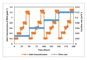
Fig. 2 Start-up of the biofilter for the removal of MEK using press mud based biofilter
