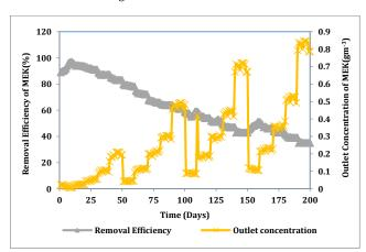
$\textbf{Fig. 3} \ \ Performance \ of \ biofilter \ for \ the \ removal \ of \ MEK \ using \ press \ mud \ based \ biofilter$
