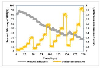
Fig. 4 Performance of biofilter for the removal of MEK using Press mud based biofilter
