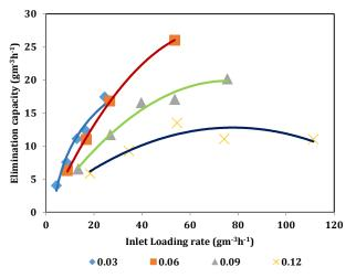
Fig. 5 Inlet Load Vs Elimination capacity for the removal of MEK using press mud based biofilter
